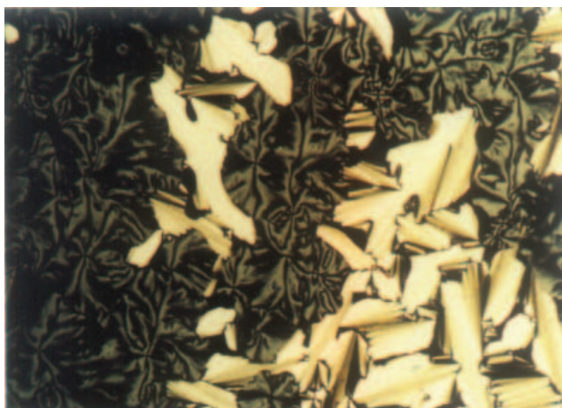
Figure 1. Photomicrograph of the SmCP A phase of compound A6 obtained on cooling the isotropic phase.
